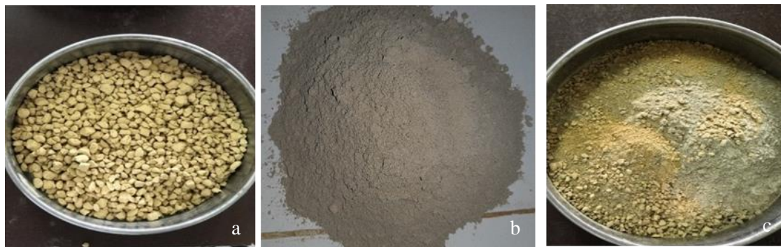
Fig. 1. Soil used: a) kaolin, b) bentonite, c) soil KB
