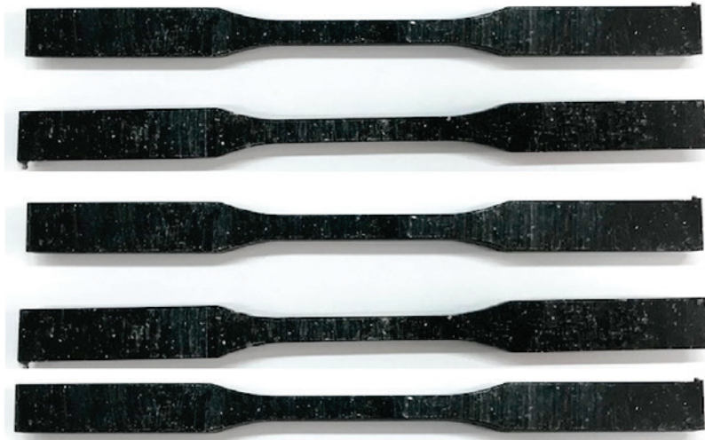
Fig. 2. Examples of samples prepared for a static tensile test
