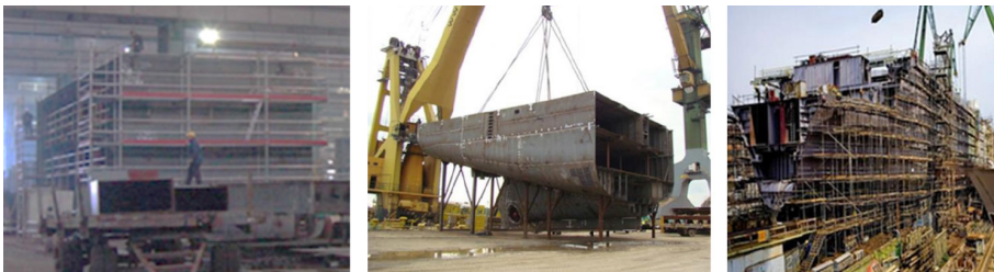
Fig. 1. Example sections and blocks of large-scale ship steel structures Source: own elaboration based on BERA et al. (2023).
