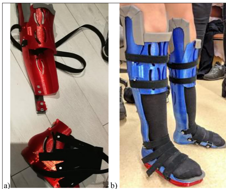
Figure 6. (a) An orthosis with a lighter design that broke during use, (b) an orthosis with a monolith construction
