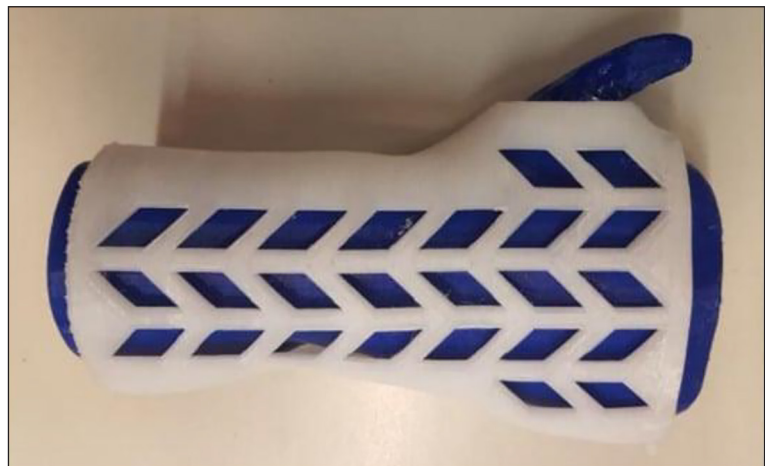
Figure 3. Orthosis on a two-material forearm phantom [13]
