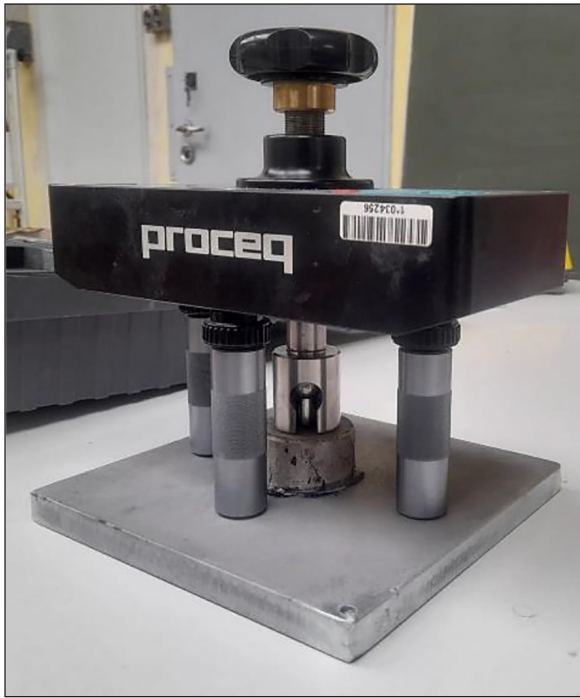
Figure 2. The test stand – OK1 series sample attached to Proceq DY-216
