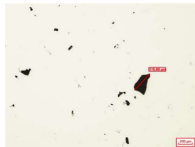
Fig. 4. Example of porosities encountered in parts produced in SLM
