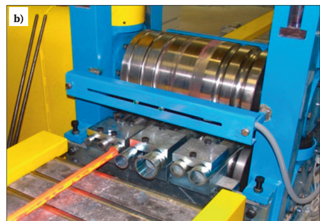
Fig. 1. Reversing duo rougher [7]
