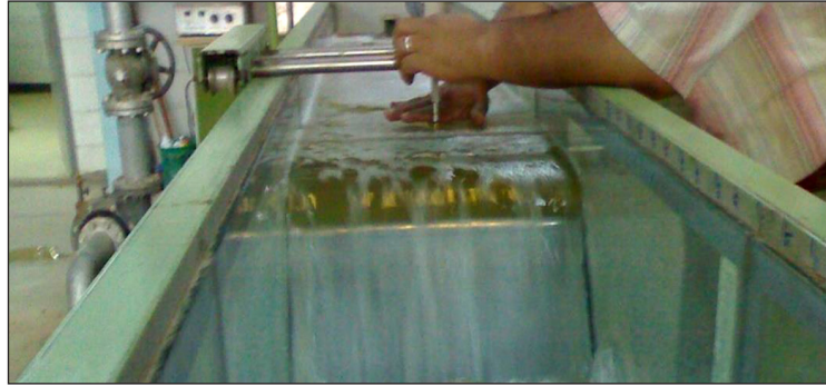
Fig. 1. General view of the laboratory channel with a broad crest weir
