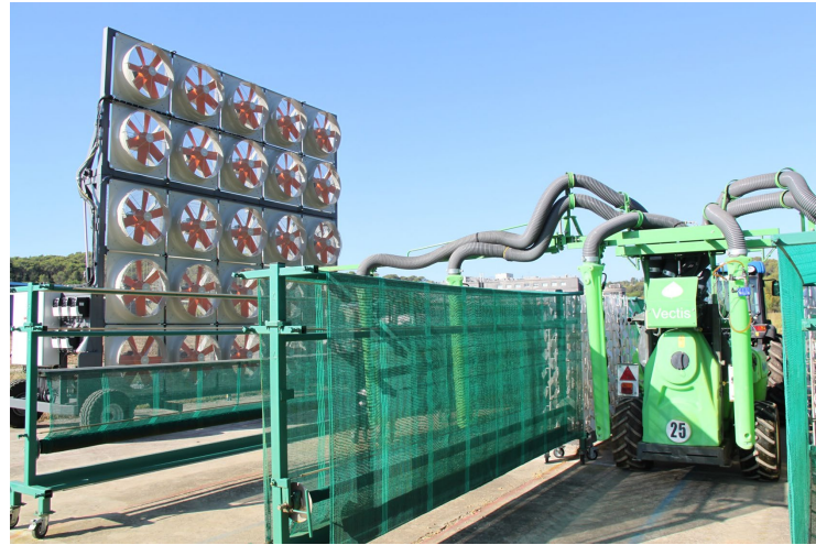
Figure 9. Potential spray drift measurement combining artificial wind and an artificial vineyard Source: UMT Ecotech, Montpellier
