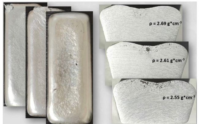
Fig. 7. View and section of representative samples with alloy density \rho = 2.55 \div 2.69 \text{ g*cm}^{-3}
