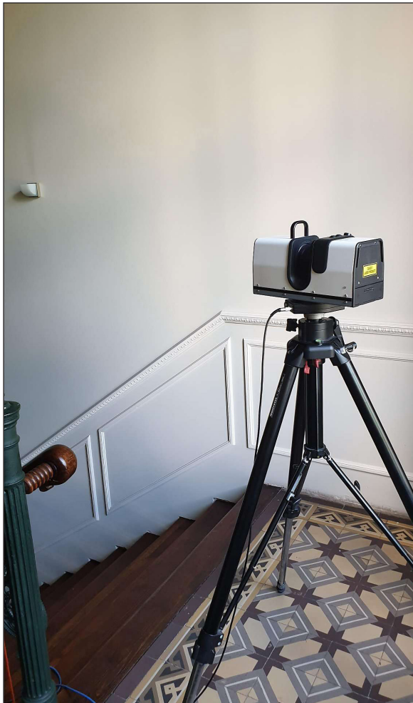
Fig. 1. Artec Ray scanner measuring the staircase
