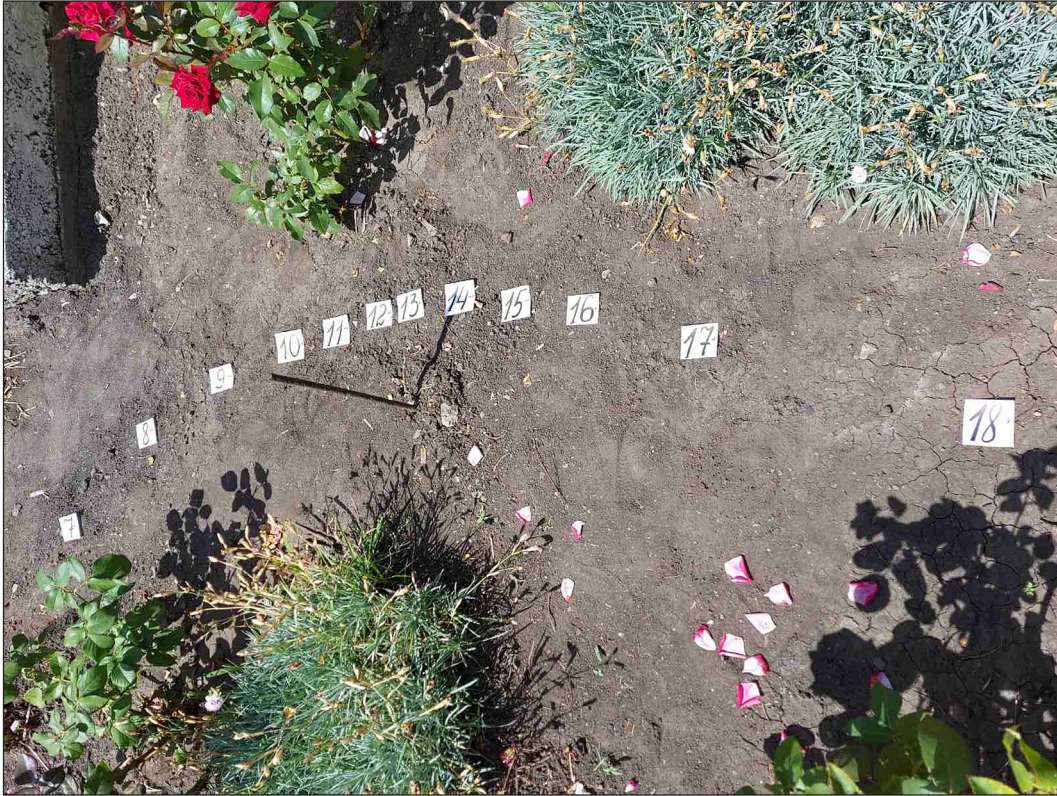
Figure 2. Position of the shadow of a gnomon with a height of 30 cm during daylight hours, the numbers indicate the hours
