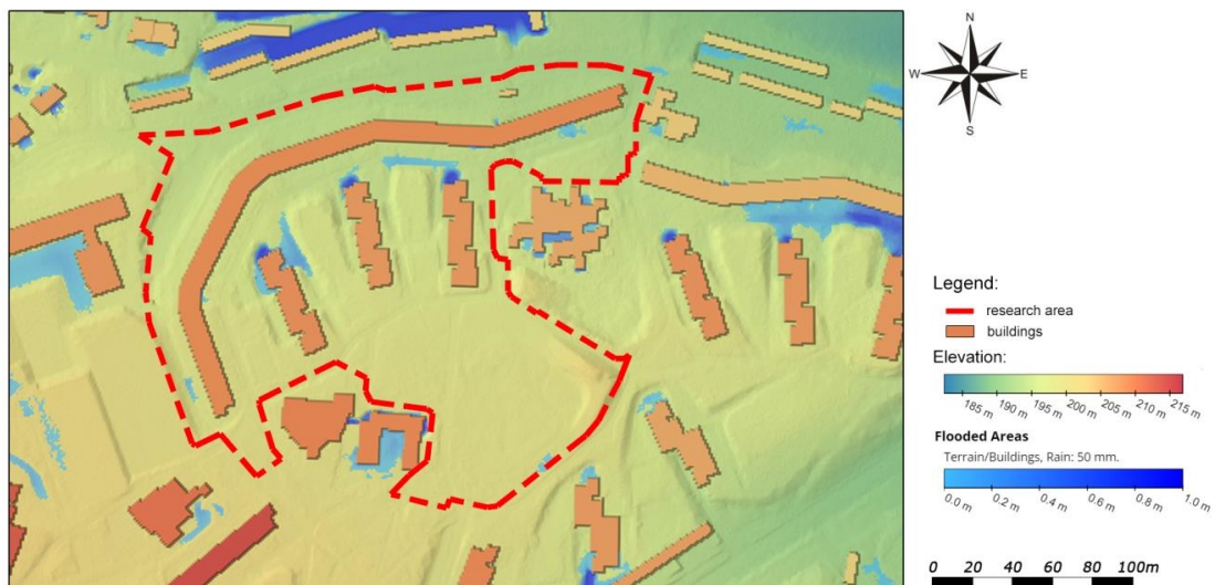
Fig. 4. Housing estate in the Rury District in Lublin. Visible areas of rainwater accumulation during heavy rainfall of 50 mm; Source: own study based on SCALGO Live.
