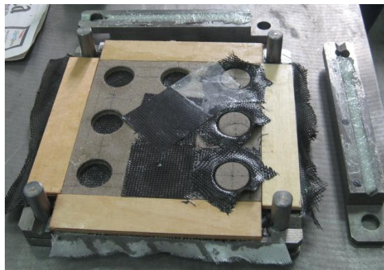
Fig. 12 Example of treatment of increasing loading abilities of sandwich structure (additional reinforcement of the foam-core)
