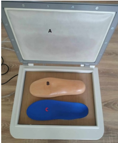
Fig. 8. System for making thermoplastic insoles. A- vacuum pump, B - last, C - ready insole. (source: own research)
