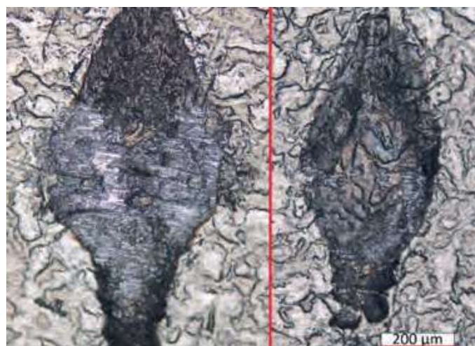
Fig. 2. Wire material remaining on the battery surface after shear test with 2 th (left) and 1 st (right) set of process parameters
