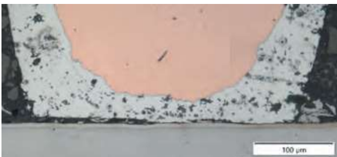
Fig. 3. Discontinuities in the interface area for the 1st set of welding parameters (200× magnification)
