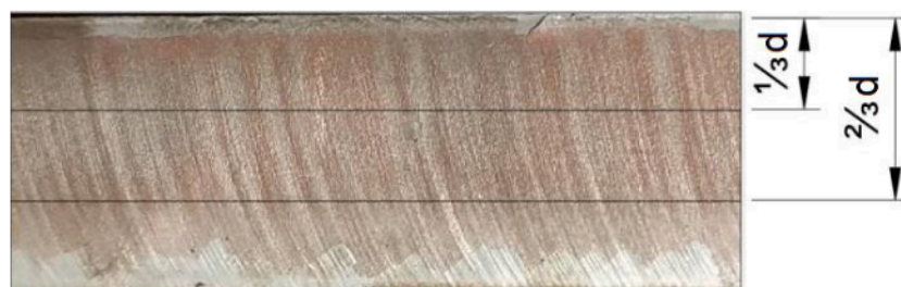
Fig. 4. Schematic of roughness measurement
