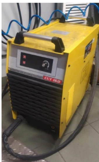
Fig. 1. MAGNUM CUT 160 plasma cutter
