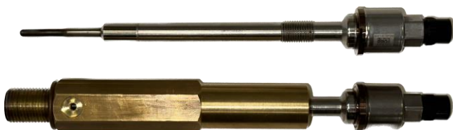
Fig. 2. PSG mounted inside the spark-plug fitting adapter next to a PSG
