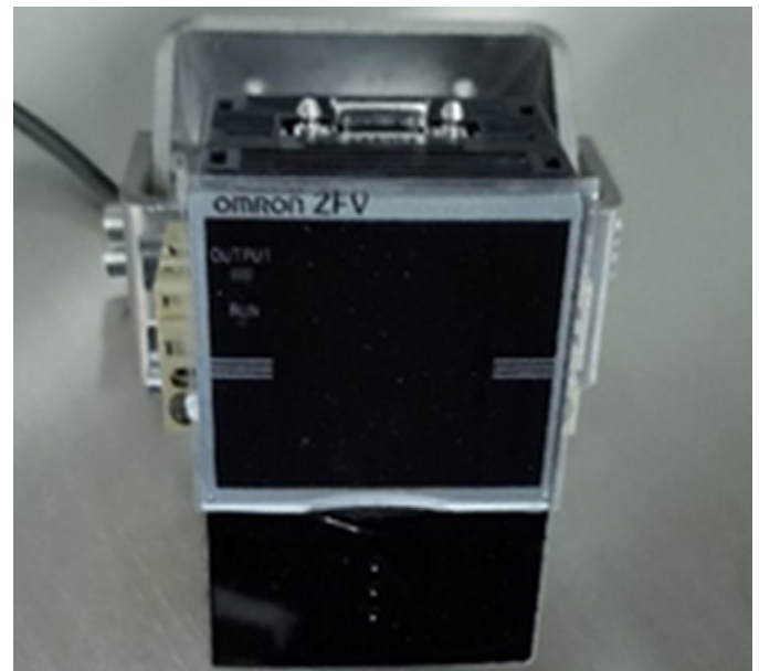
Photo 3. Camera setting panel assembled with adjustable mount
