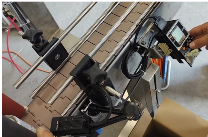
Photo 6. Calibration of the camera in the image from the label
