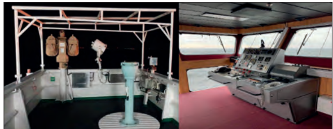
Fig. 2. Example of workstation for docking on open wing (left) and on totally enclosed wing (right)
