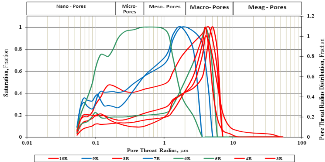
Fig. 9. Pore throat size distribution for studied Baharya reservoir samples.
