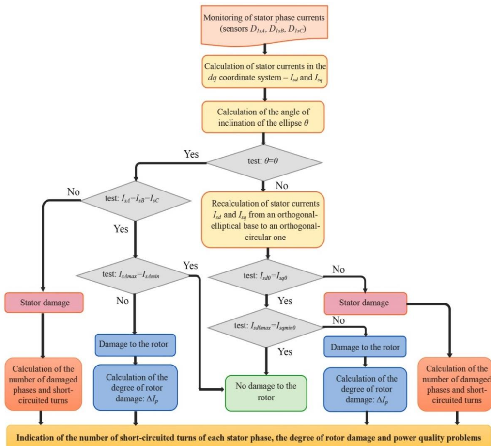
Fig. 4. Algorithm of the modular unit for monitoring the state of the stator and rotor windings of asynchronous machine (author's development)
