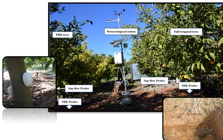
Figure 2. Photo of the experimental station with the measurement probes
