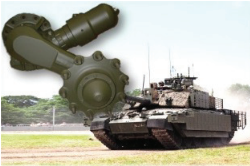
Fig. 3. Challenger tank hydropneumatic spring
