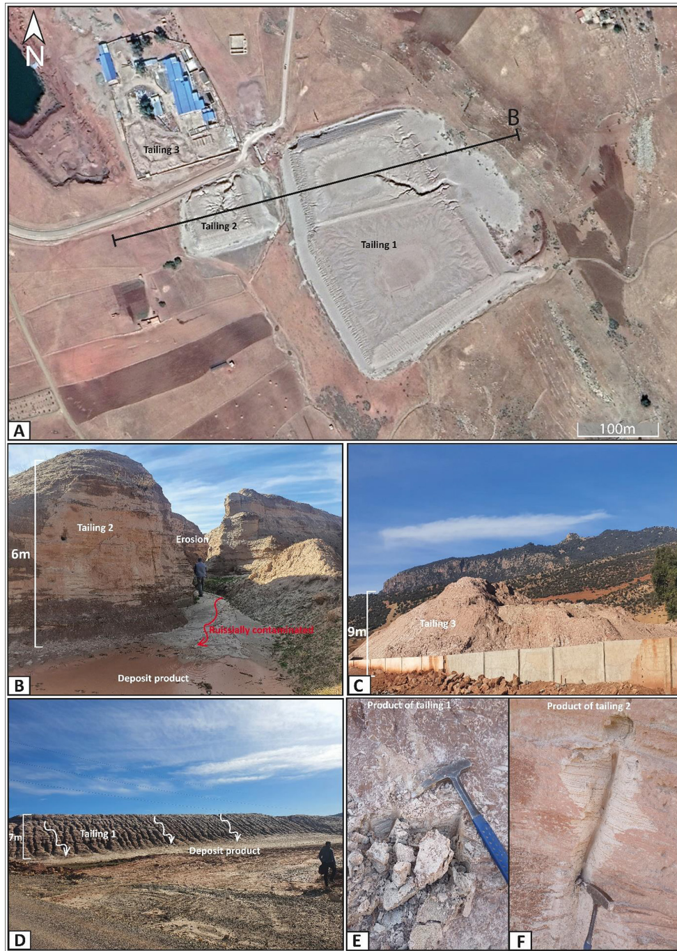
Figure 3. Mine tailings from the Tansrift mine; (a) Erosion and run-off from mine tailings 2; (c) The third mine tailings with their erosive aspect; (d) The first mine tailings with their erosive aspect and products in the surrounding soils; (e) Mine residues from mine tailing No. 1; (f) Products from mine tailings No. 2
