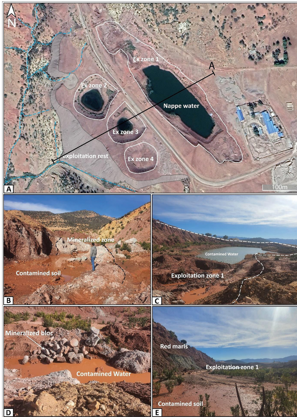
Figure 2. The Tansrift mine exploitation area; (a) the mine exploitation areas (Google earth); (b) the mineralized structure hosted in sandstone; (c) the exploitation reaches the contaminated water table; (d) natural leaching product of mine tailings; (e) contaminated soil in the mine exploitation area
