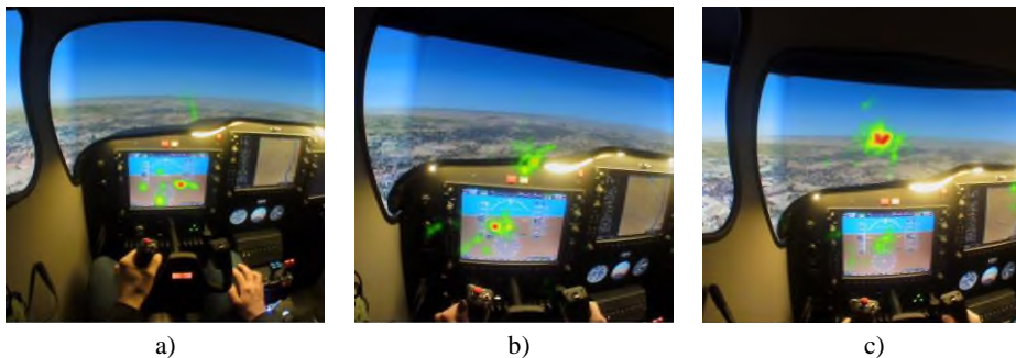
Fig. 2. Heatmaps of pilots (a) expert, b) intermediate and c) novice) performing the first landing approach
