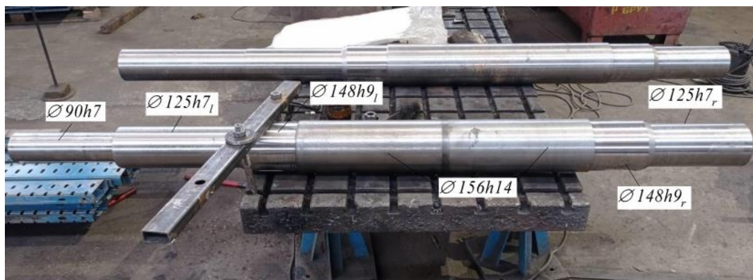
Fig. 6. Conveyor belt drive drum shaft.
