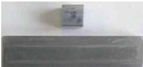
Fig. 5. Sample – GJL-250+Cr- \text{Al}_2\text{O}_3 (top) and counter-sample AC-47000+15% \text{Al}_2\text{O}_3 (bottom) after tribological tests
