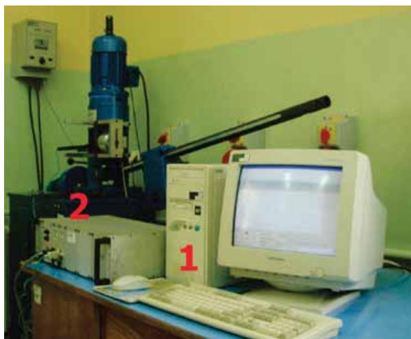
Fig. 1. Test stand for measuring lubricity properties: 1 – personal computer for the test control with appropriate software installed 2 – 4-ball apparatus with a digital amplifier and a set of measuring transducers (Poland)
