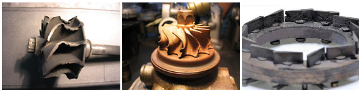
Fig. 2.9. Damage following penetration of a foreign object into the turbine
