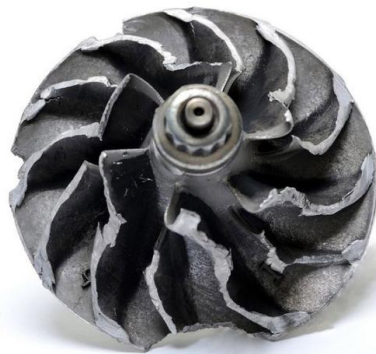
Fig. 2.5. Damage to the compressor vanes caused by excessive shaft play
