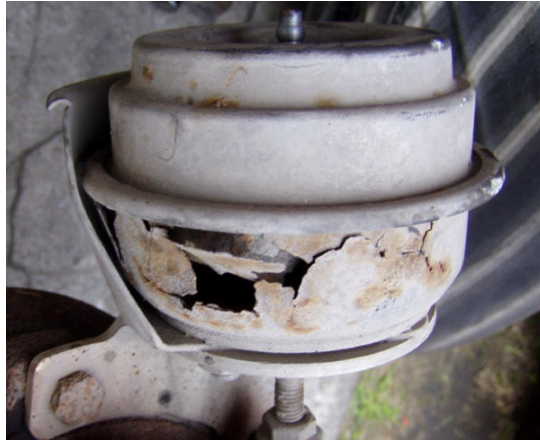
Fig. 2.14. Corroded pressure adjuster of the turbocharger in Skoda Octavia
