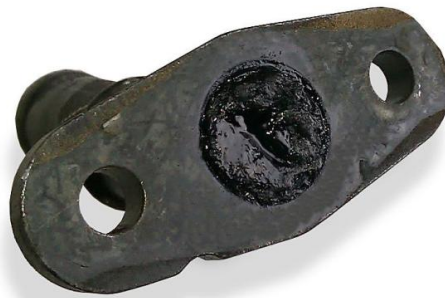
Fig. 2.12. The result of overheating – congested (by oil originating carbon deposits) turbocharger drain duct
