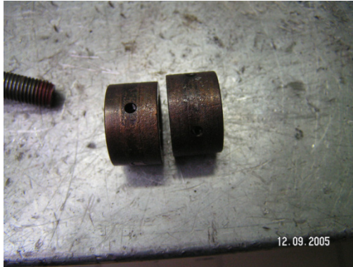
Fig. 2.6. Seized and damaged surfaces of the bearings
