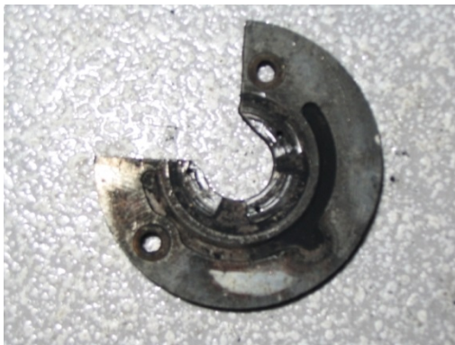
Fig. 2.7. Overheated longitudinal bearing and seized surface of the turbocharger shaft
