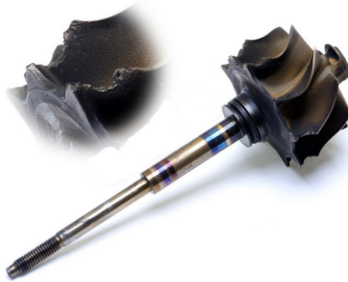
Fig. 2.13. Chipped and melted turbine rotor vanes because of high exhaust gas temperature
