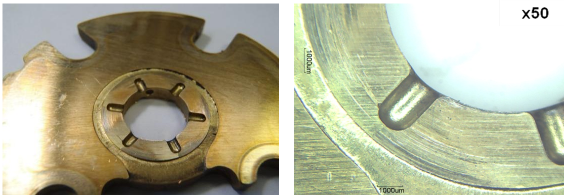
Fig. 2.2. Scratches of longitudinal bearings
