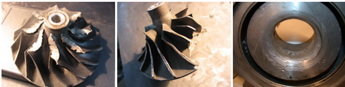
Fig. 2.8. Damage following penetration of a foreign object into the compressor
