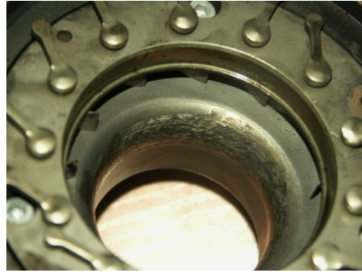
Fig. 2.4. Damage of the body surface on the side of the turbine
