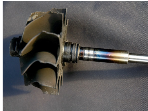
Fig. 2.7. Overheated longitudinal bearing and seized surface of the turbocharger shaft
