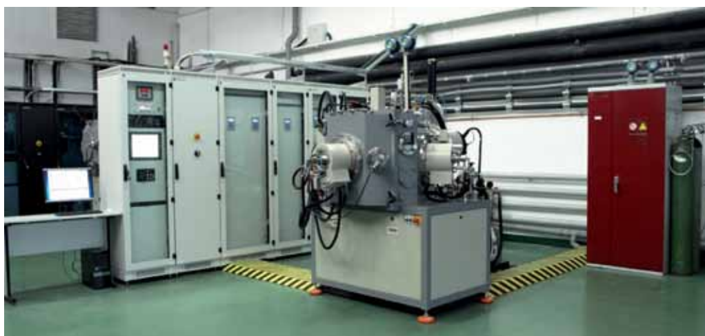
Fig. 1. Plasma reactor used for surface modification of polypropylene designed and built at ITeE – PIB in Radom (Poland)
