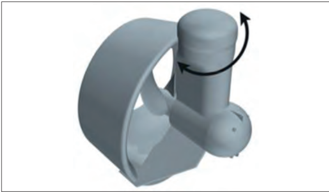
Fig. 8. Yaw angle about vertical axis
