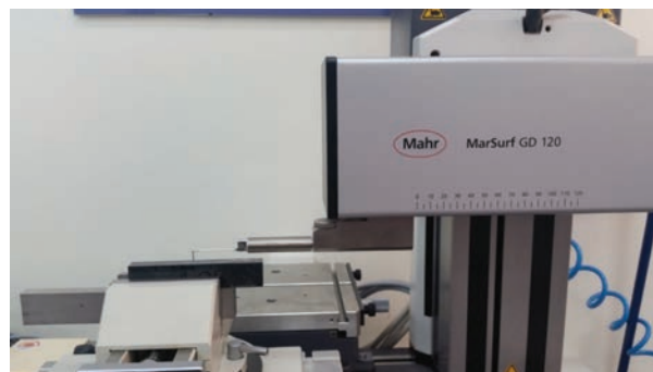
Fig. 2. A sample photograph of the roughness measurement
