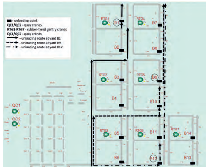
Fig. 7. Layout of the seaport terminal, showing three exemplary discharge routes considered in the simulations under Routing Strategy 2
