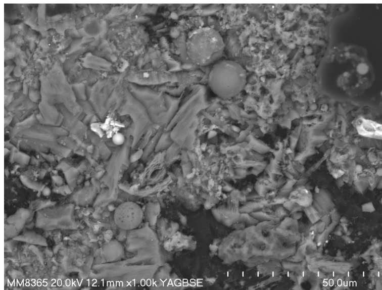
Fig. 5. Gypsum crystals in black crust. Spherical aluminosilicate dust particles; bright particle is rich in Fe. SEM, BSE image
