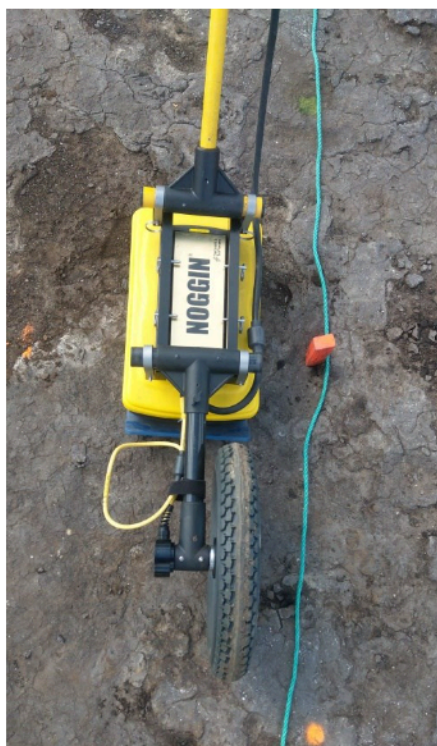
Fig. 1. GPR Noggin with 500 MHz antenna
