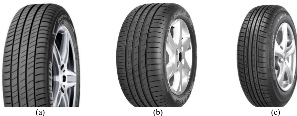
Fig. 5. Tires of the cars included in the experiments: (a) Michelin Primacy 3 215/55 R18, (b) Goodyear 215/50 R17, and (c) Dunlop sport Fast response
