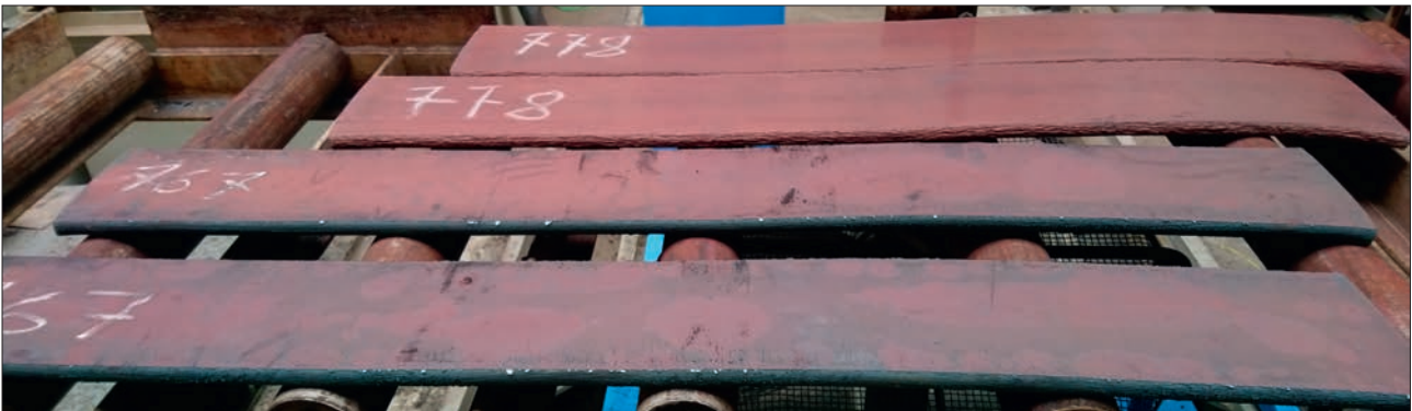
Fig. 2. Photograph of flat bars from the tested materials after rolling in LPS-B into strips with a final thickness of approx. 17 mm
