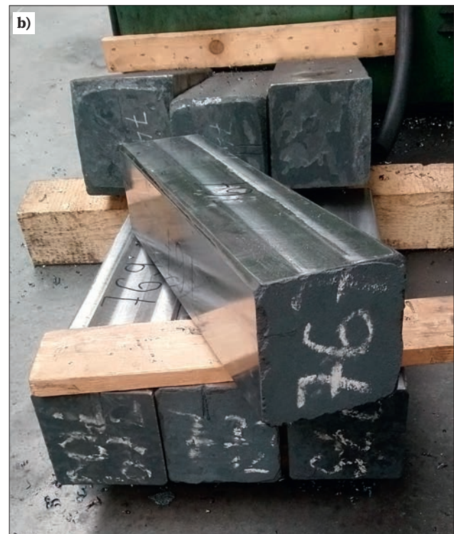
Fig. 1. Photographs of laboratory ingots after homogenisation annealing (a) and surface milling (b)
