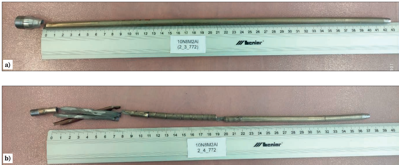
Fig. 7. 10N8M2Al steel bars after hydrostatic extrusion with strain a) \epsilon = 1.53 , b) \epsilon = 1.8 [15]
