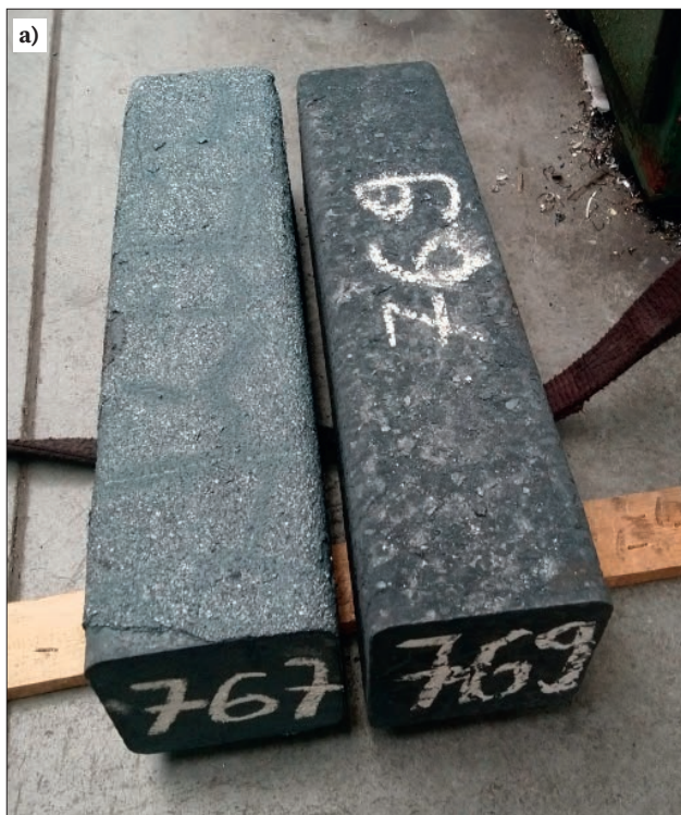
Fig. 1. Photographs of laboratory ingots after homogenisation annealing (a) and surface milling (b)
