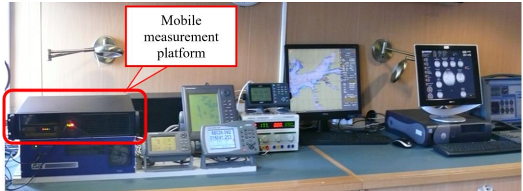
Fig. 13. Mobile measurement platform with external navigation devices providing the necessary measurement data (source: own study)
