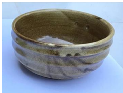
Fig. 1. The application of glaze ceramics based on basalt from the Bali Province
