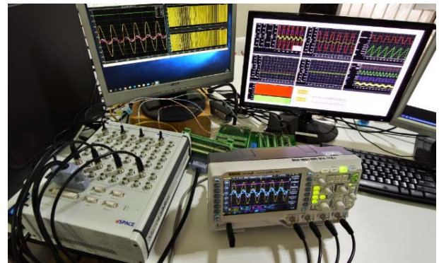
Fig.13 The installation of the HIL testing equipment
