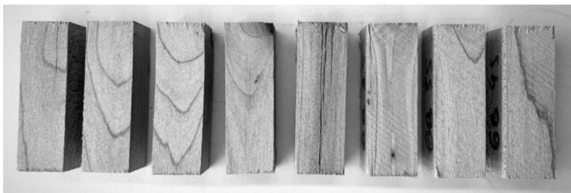
Figure 14. Samples squeezed as a result of wood compression strength test of red maple on the N-S axis of tree no.6.
