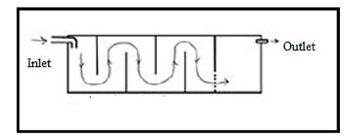
Fig. 2. Top view of the constructed wetland.
