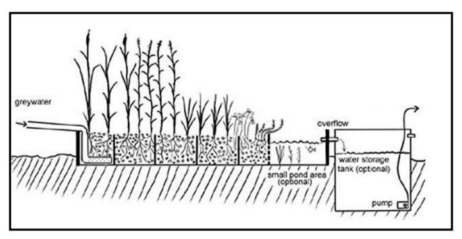
Fig. 1. Simplest schematic flowdiagram of constructed wetland.
