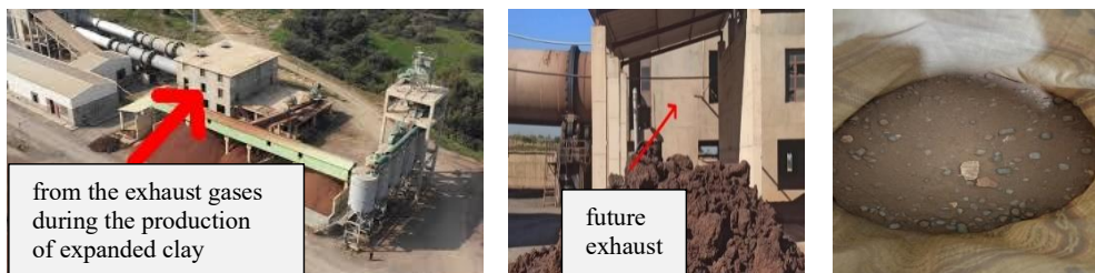
FIGURE 2. Source of expanded clay kiln dust (ECKD) raw material
