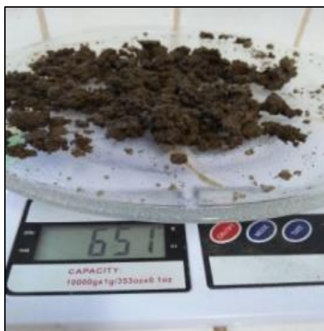
Sample was weight and reheated for 5 minutes, until the weight is constant.
