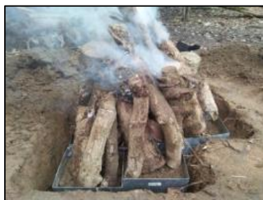
LM 1 and LM 2 in the earth pit with woods placed and set fire above, for pyrolysis
