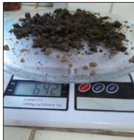
Sample was weight and reheated for 5 minutes, until the weight is constant.
