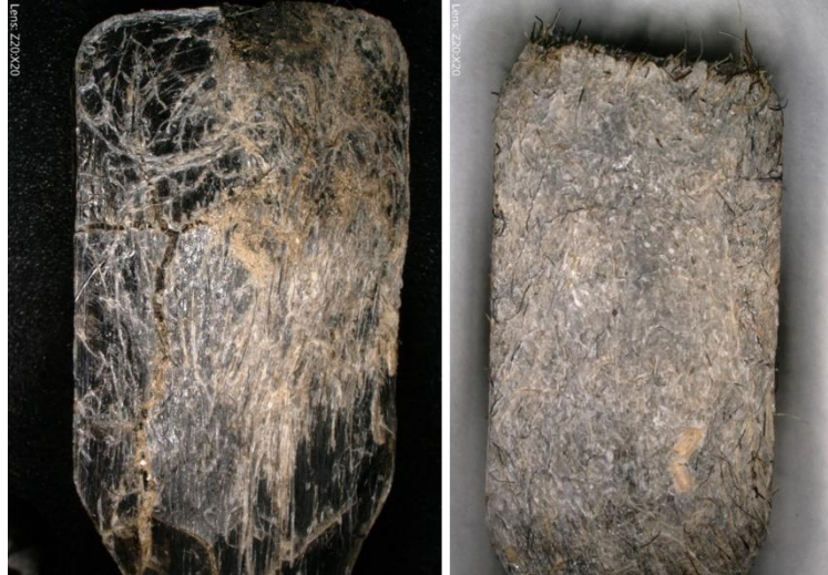
Photo 2. Advancement of the biodegradation process in wool/PLA sample subjected to 48-h ageing in the ageing chamber (left G7, right G8)
