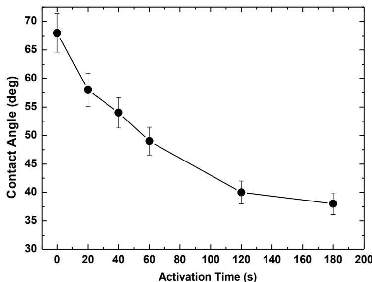
**Figure 5.** Contact angle of water on beech wood surface modified by RF discharge plasma vs. activation time.
