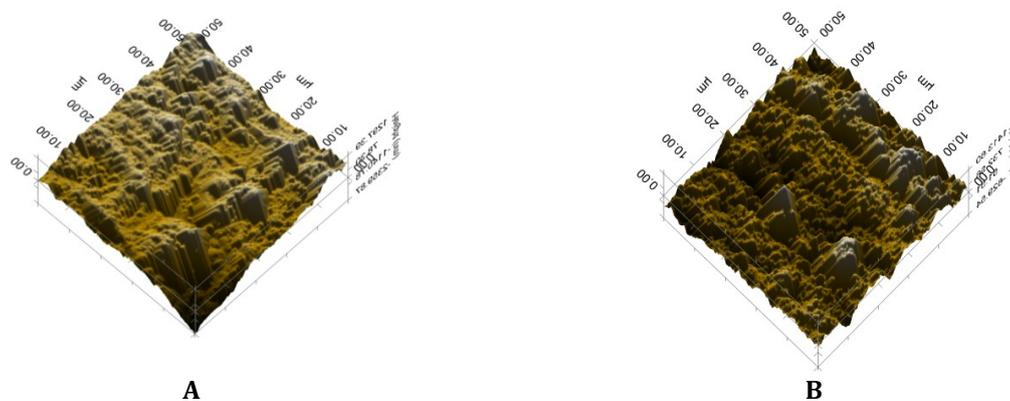
**Figure 3.** Nanoindentation analysis of beech wood: A – pristine sample, B – CCRF plasma modified sample, 120 s (50×50 nm).
