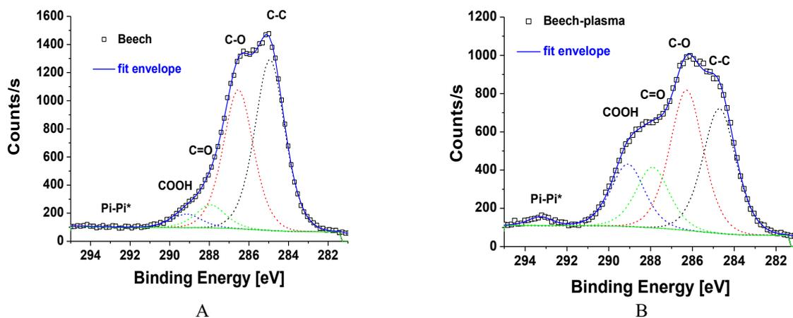
**Figure 4.** XPS spectra of beech wood modified by RF plasma (120 s): A – carbon C1s peak of pristine beech wood, B – carbon C1s peak of plasma-treated beech wood.
