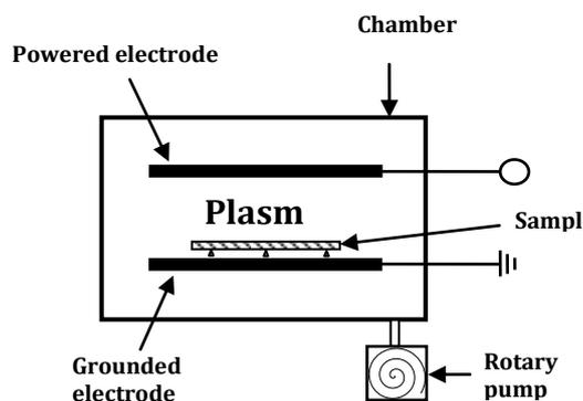
**Figure 1.** Scheme of RF discharge plasma source
