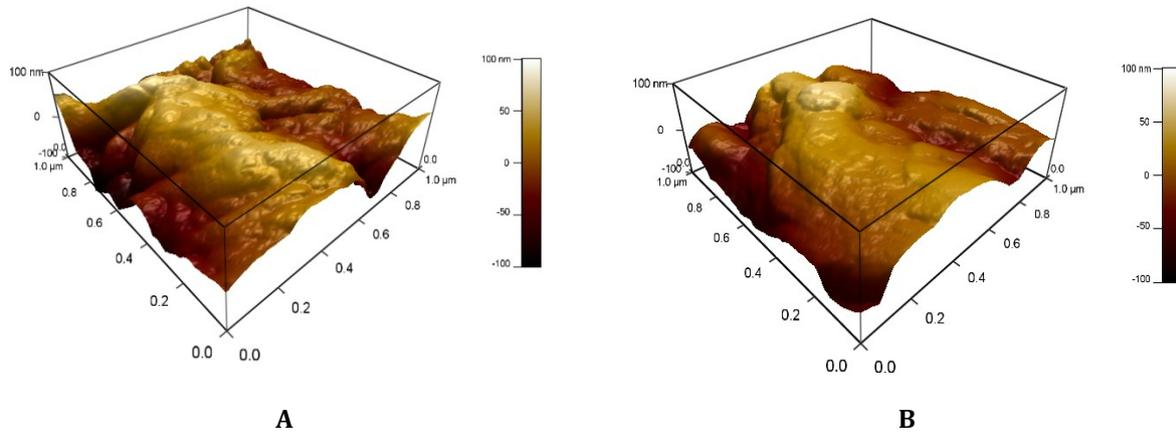
**Figure 2.** 3D AFM images of beech wood: A – pristine sample ( $R_a = 21.8$  nm), B – RF plasma-treated sample ( $R_a = 18.7$  nm), 120 s (1000×1000 nm).
