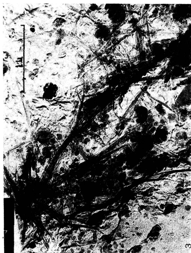
Plate I. Fig. 1. Doubly refractive streaks are clearly seen. Thin section under crossed polarizers. Sample 1; \times 130 . Fig. 2. Plasma dominant over skeleton grains. Thin section. Sample 6; \times 130 . Fig. 3. Sepiolite fibers crossed among themselves showing a trend towards a fluidal disposition. Replica technique. Sample 1; \times 30,800 . Fig. 4. Abundance of kaolinite intermixed with goethite. Normal dispersion technique. Sample 6; \times 37,600 .
