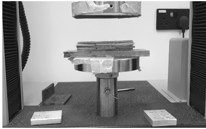
Fig. 2. Applying clamping pressure on a 5 layer specimen using a UTM
