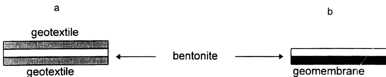
Fig. 4. Cross section of current available GCLs
